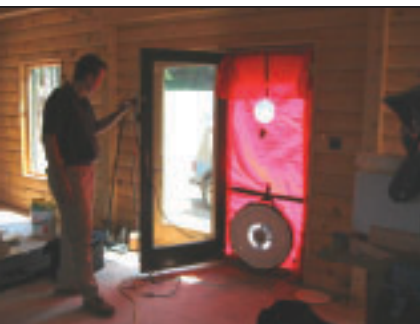
Eight of Alta's log homes have earned Energy Star certification. Blower door tests are key to the HERS scoring.
